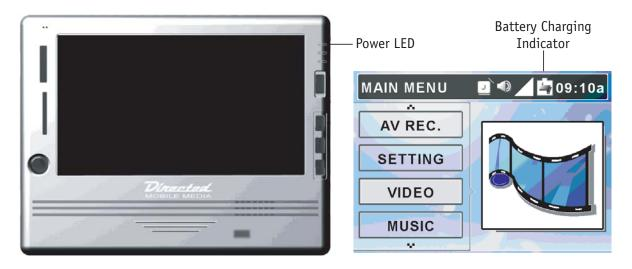
3. When the battery is fully charged, the Power LED will stop flashing and the charge indicator on the battery icon will disappear. Disconnect the AC Adapter from the player.
